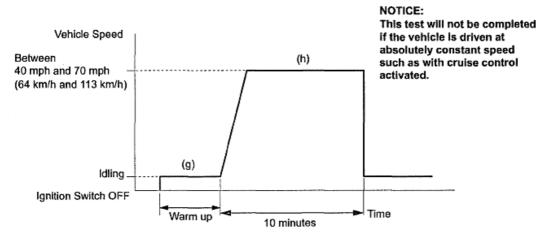
(Note: Even if vehicle stops during driving pattern, test can be resumed)
